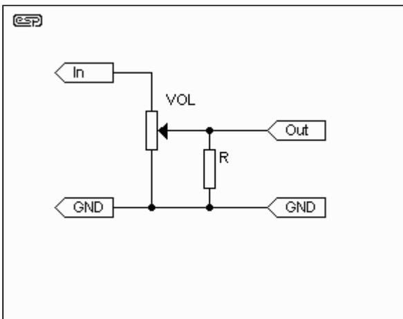
Figure 1 - Circuit of the Log Pot Approximation
