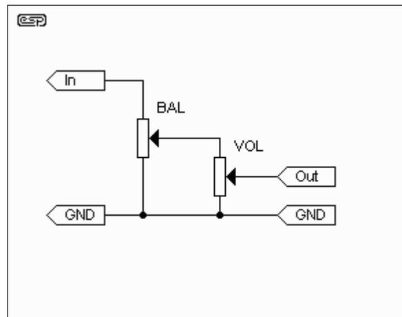
Figure 4 - Conventional Balance / Volume Control
