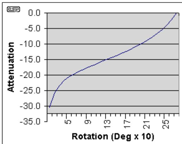
Figure 2 - The Transfer Curve in dB
