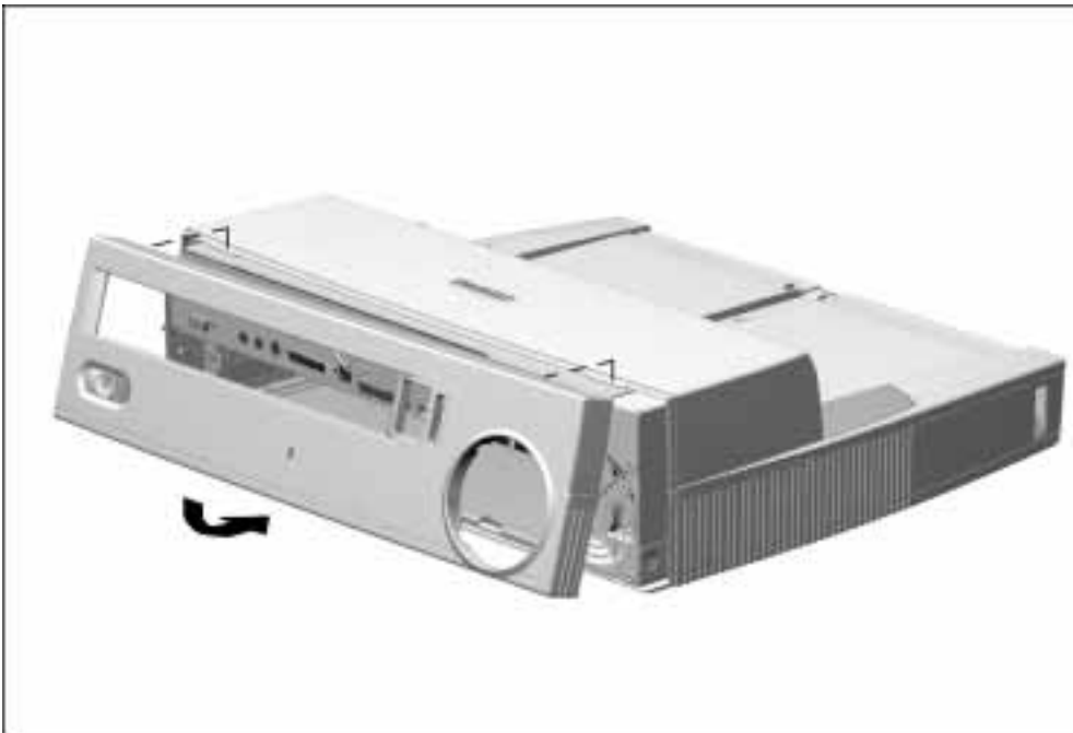
Figure 5-10. Installing the Rear Panel Assembly
