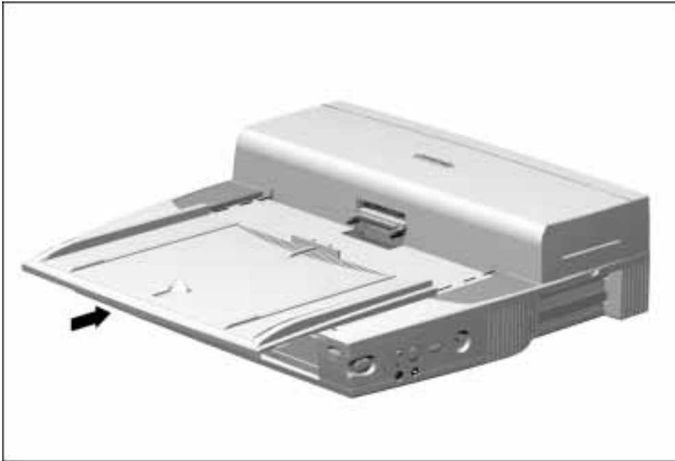
Figure 5-7. Installing the Alignment Tray Assembly
